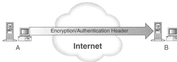
Figure 6–3: A pair of hosts using IPsec to communicate transparently across the Internet.
