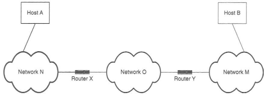
Figure 5-3: Dual-stack systems can interoperate with IPv4 and IPv6 nodes.
