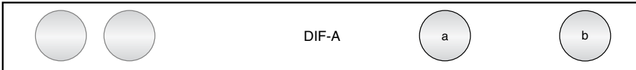
Figure 7-11 A new system has just joined the network, been authenticated, and assigned an (N)-address and is now ready to participate as a member of the DIF.
