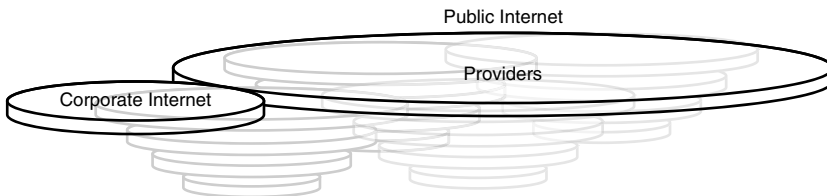
Figure 8-10 The public Internet is just another “top” layer that applications may access. It is supported by multiple providers, as is a corporate network.
